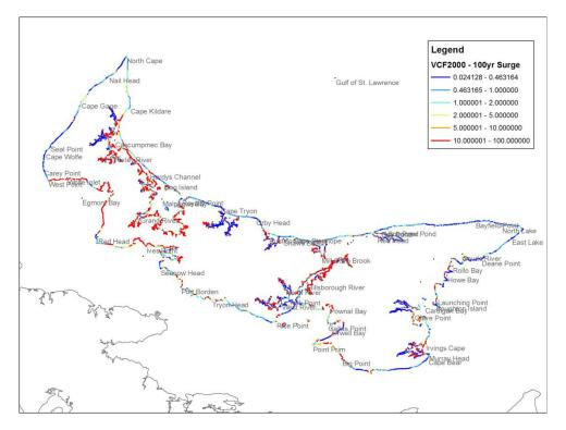
Figure 56 Vulnerability to Coastal Flooding (100-year surge, mean sea level in 2000).
